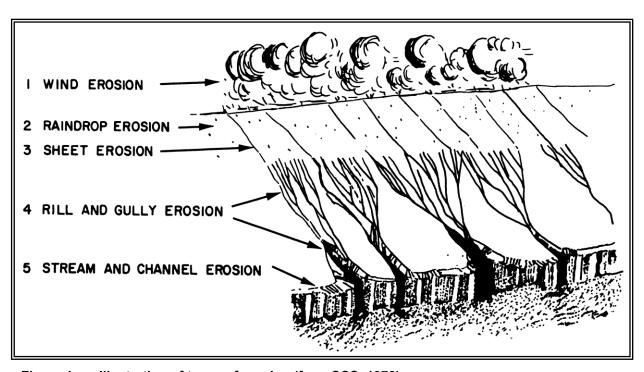
Figure 1 Illustration of types of erosion (from SCS, 1978)
