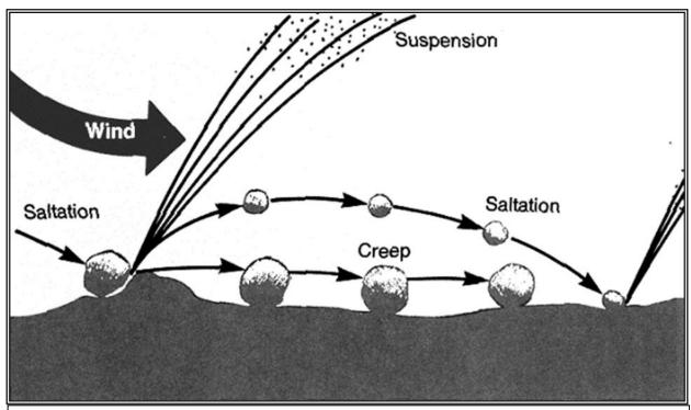
Figure 2 Mechanisms of erosion and sediment transport by wind (from SCS, 1989)
